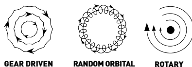
GEAR DRIVEN RANDOM ORBITAL ROTARY
